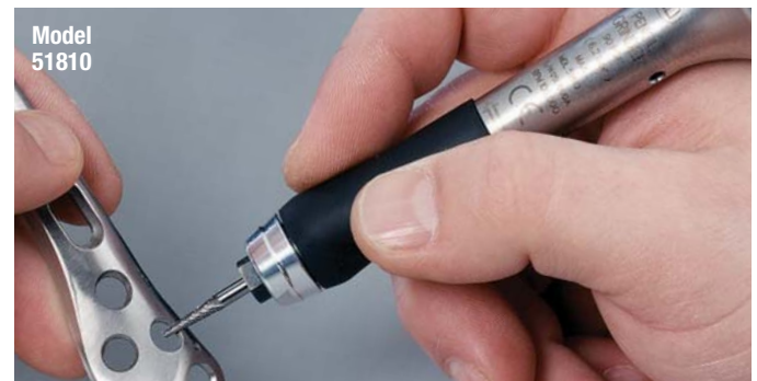
100,000 RPM Pencil Grinder offers enhanced cut rate.
