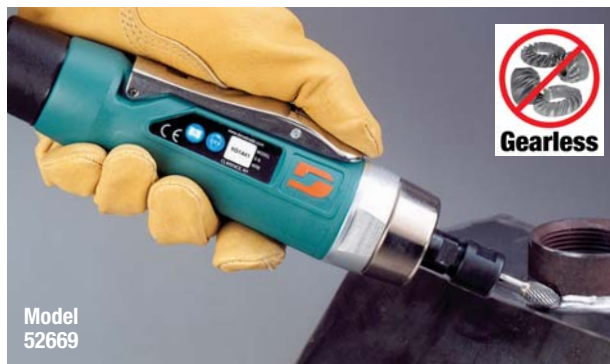
Use a carbide burr to easily blend weld seams.
