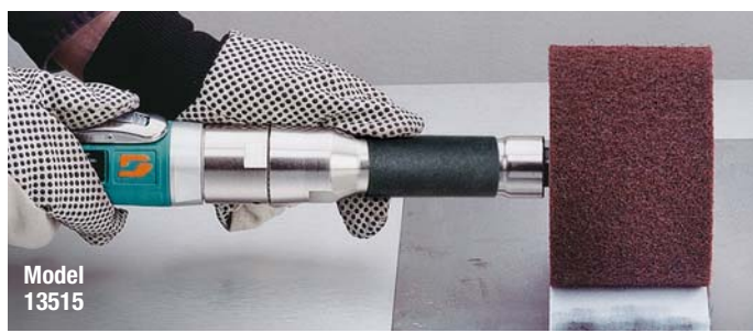
13515 Dynastraight® sets grain pattern in stainless steel.
