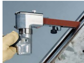
15400 Dynafite® III allows finishing and deburring in restricted areas.
